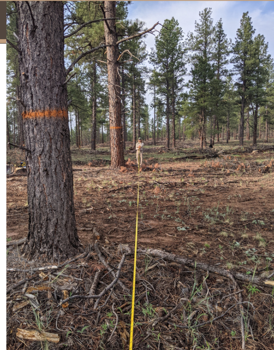
Figure 1: a researcher determines azimuth of a line while laying out a forest inventory transect.
