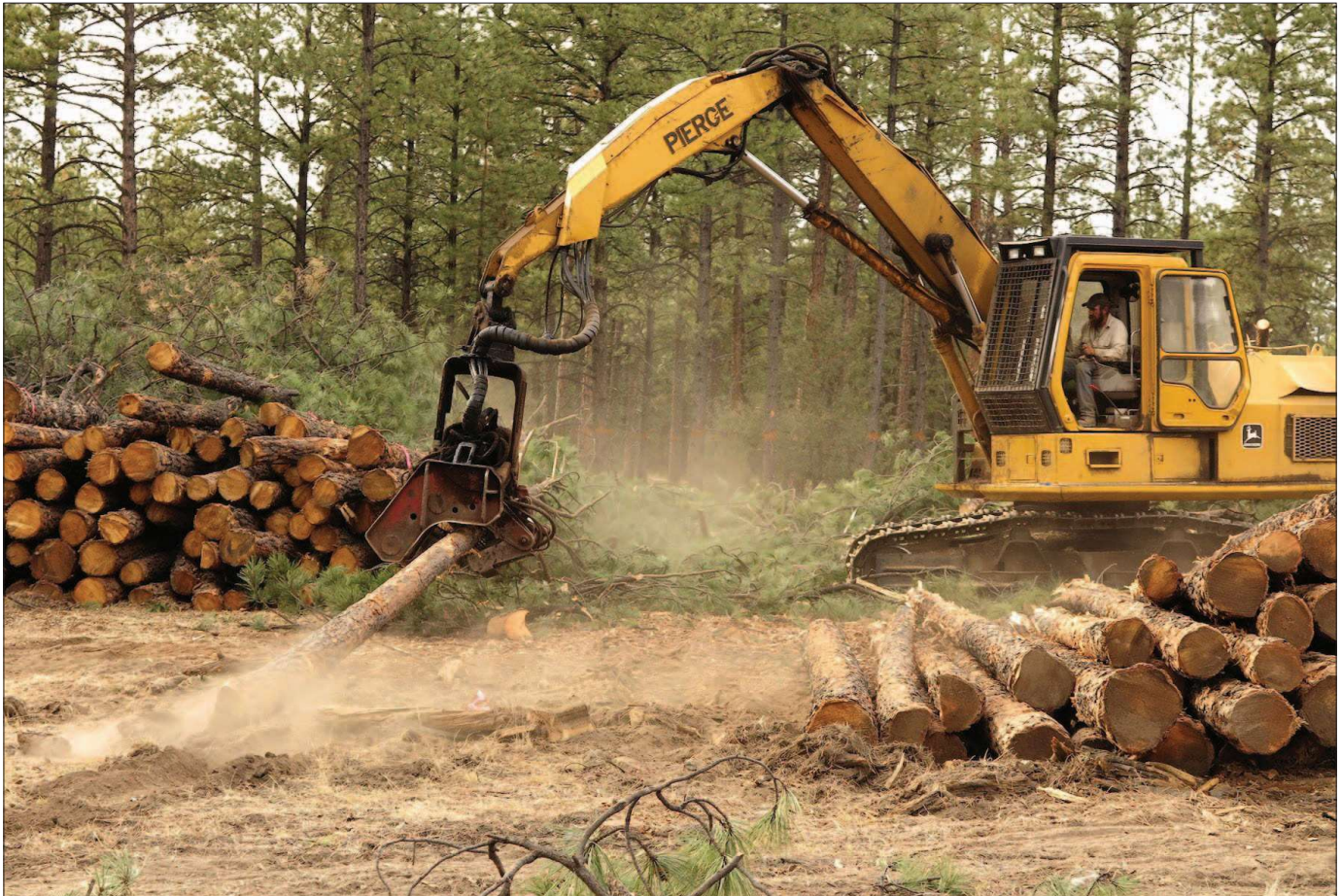
A delimeter processes ponderosa pine logs destined for Mt. Taylor Manufacturing, a sawmill in Milan, New Mexico, that produces dimension lumber, cants, wood pellets, playground chips, animal bedding, and other products.
